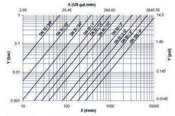
Medium: Water, 20 °C X flow rate l/min], (US gal./min) Y pressure loss Δp (bar), (psi)
