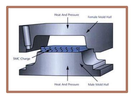
While the mould remains closed, the thermosetting material undergoes a chemical change (cure) that permanently hardens it into the shape of the mould cavity. Mold closure times vary from 30 seconds up to several minutes depending on part design and material formulation.
