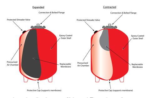
increases the membrane inside the vessel expands to allow the water to fill the vessel. The membrane will continue to expand until the system reaches its maximum temperature.
