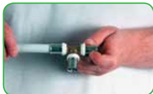
Insert pipe in to fitting until pipe is visible in hole of sleeve
