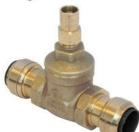
Brass full way gate valve with lockshield. Tectite push-fit ends for copper, carbon and stainless steel tube.
