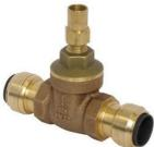
Bronze full way gate valve with lockshield. Tectite push-fit ends for copper, carbon and stainless steel tube.
