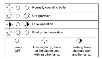
If the lights sequence observed on the boiler is not included above then a fault is indicated.
