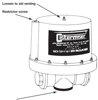
Sensitivity adjusting screw beneath knurled brass sealing cap. Turn anti-clockwise to increase sensitivity.
