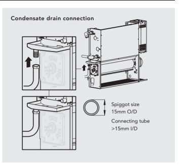
A drain tray is fitted for condensate collection within the unit. This should be connected to a 15mm drain pipe.
