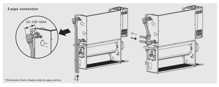
Note 1: The flow pipe should be connected to the bottom connection of the heat exchanger.
