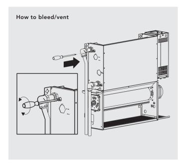
Ensure all water fittings are secure before filling the heating
