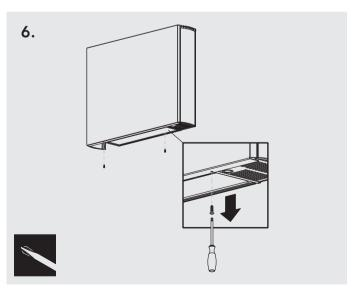
NOTE: Do not replace outer cover until connection to system and connection to electrical supply has been completed.
