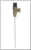
AQ1 Pressure and temperature relief valve (7 bar/90°C). Provides additional levels of safety when fitted to water heater as shown in Diagram D. Note: Varipoint supplied complete with AQ1. Order AQ1 separately for use with Aquapoint.
