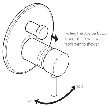
Moving the contol lever anti-clockwise will decrease the water temperature. Pull the handle out to increase the flow of water.
