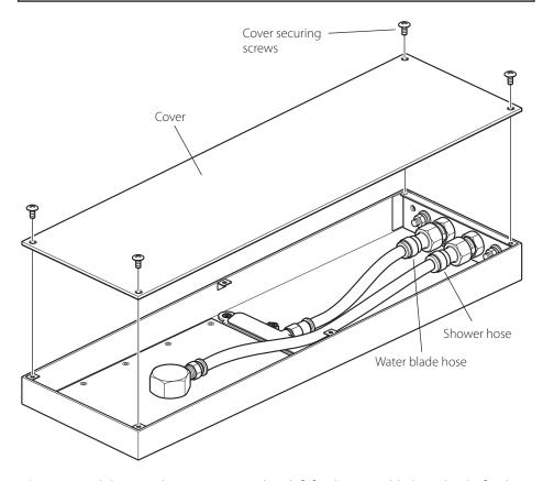
Connect each hose to the connecting tubes, left for the water blade and right for the shower.
