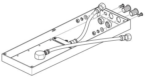
Slide the body over the bolts and connectors. Slide on a plain washer a spring washer and a nut onto each fixing bolt and tighten, before finally tightening check for level, when satisfied tighten down the bolts.
