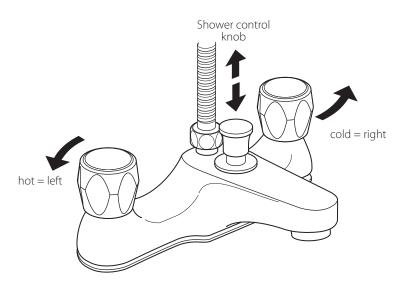
Moving the control handles anti-clockwise will increase the flow of water.
