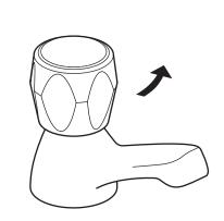
Hot tap - turning the control handle anti-clockwise will increase the flow of water.
