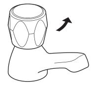
Cold tap - turning the control handle anti-clockwise will increase the flow of water.
