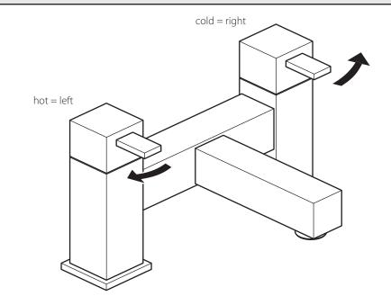
Moving the levers in the direction of the arrows will increase the flow of water.
