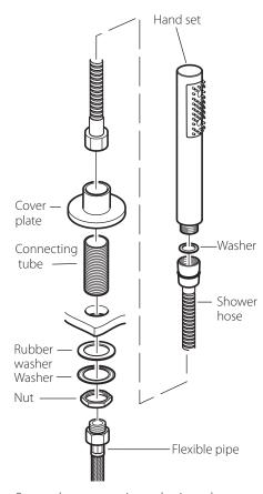
Screw the connecting tube into the cover plate and position in the hole, from the underside slide on the rubber washer, metal washer and then the nut. Tighten the nut to clamp on the cover plate.
