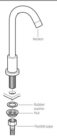
Position the spout in place, and from the underside slide on the rubber washer, and then the washer/nut. Tighten the nut to clamp on the spout.
