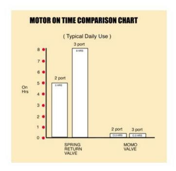
The valve has a removable actuator, which allows replacement without system drain down. Because the valve is "on" only when the valve is changing position it offers a 30% reduction in energy consumption over a traditional spring return valve.
