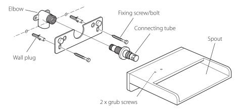
Before installing your new spout, flush through the pipework to ensure removal of debris, turn off the water supply.
