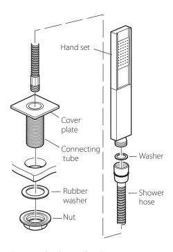
Position the Cover plate/connecting tube in place and from the underside slide on the rubber washer and nut. Tighten the nut to clamp on the cover plate.
