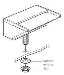
Position the spout in place, and from the underside slide on the rubber washer and nut. Tighten the nut to clamp on the spout.
