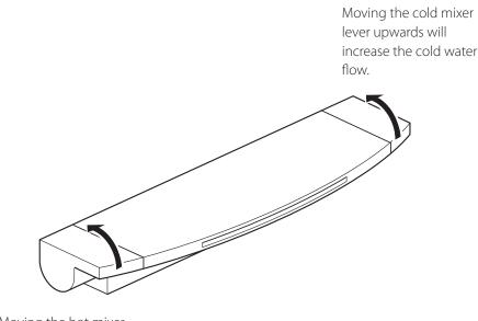
Moving the hot mixer lever upwards will increase the hot water flow.
