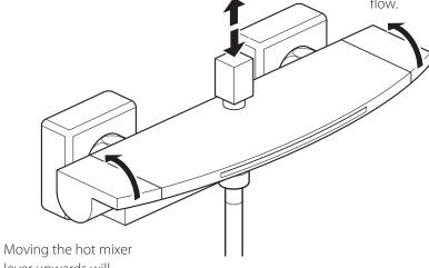
lever upwards will increase the hot water flow.
