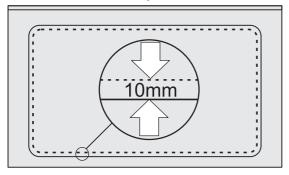
This is the cutting line for the aperture.
