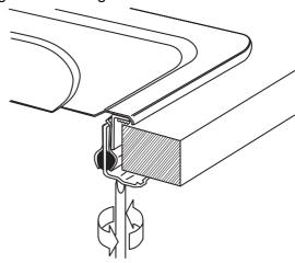
Do not overtighten the fixing clamps once the sink is fully bedded in the sealing tape. Do not tighten fully at the first attempt.
