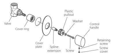
Before installing your new tap, flush through the pipework to ensure removal of debris, turn off the water supply.
