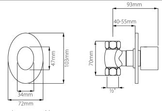
Minimum operating pressure - 1 bar Maximum operating pressure 5 bar
