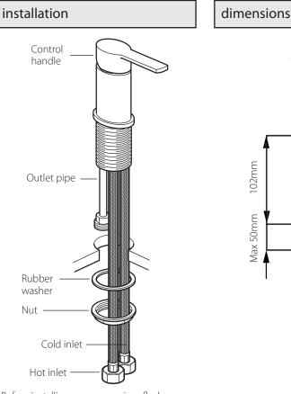
Before installing your new mixer, flush through the pipework to ensure removal of debris, turn off the water supply. Remove the nut and washer and push the valve down through the hole in the unit, slide the rubber washer and nut over the flexible pipes and outlet pipe and screw onto the valve.
