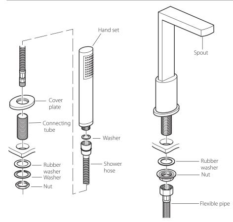
Screw the connecting tube into the cover plate and position in the hole, from the underside slide on the rubber washer, metal washer and then the nut. Tighten the nut to clamp on the cover plate.
