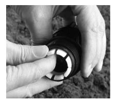
Disassembly Take the Metric/Imperial<sup>™</sup> fitting and remove the nut. The split collet and seal ring must then be removed.
