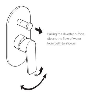
Moving the control lever anti-clockwise will decrease the water temperature.
