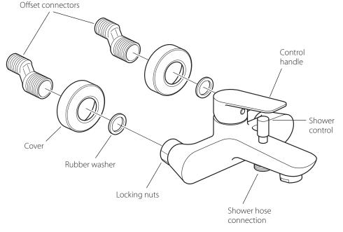
Before installing your new mixer, flush through the pipe work to ensure removal of debris, turn off the water supply.
