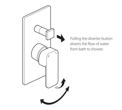
Moving the control lever anti-clockwise will decrease the water temperature. Pull the handle out to increase the flow of water.
