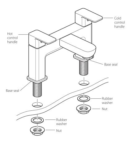
Before installing your new mixer, flush through the pipework to ensure removal of debris, turn off the water supply.
