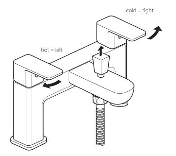
Moving the levers in the direction of the arrows will increase the flow of water. Pull the diverter knob up to turn on the shower.
