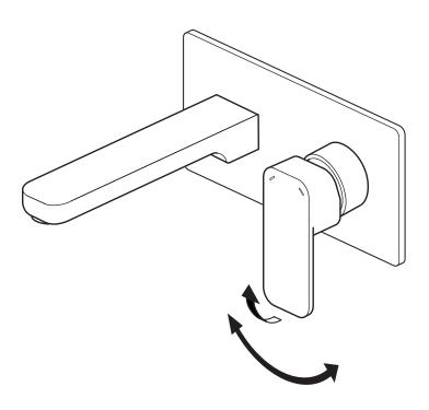
Moving the control lever anti-clockwise will decrease the water temperature.
