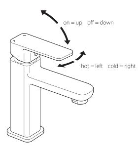
Moving the mixer lever upwards/downwards will increase/decrease the flow of water. Moving the mixer lever from right to left will increase the water temperature.
