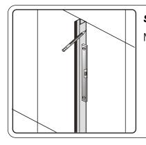
step 2. Make sure wall profile is upright using a spirit level.
