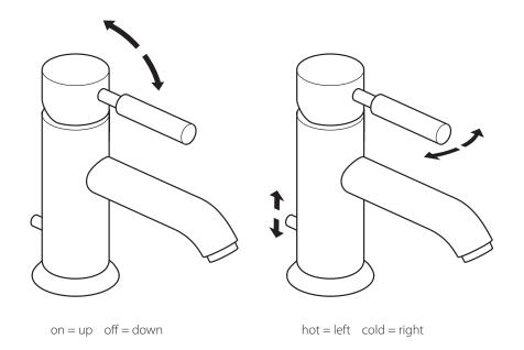
Moving the mixer lever upwards/downwards will increase/decrease the flow of water. Moving the mixer lever from right to left will increase the water temperature. Pull the vertical control rod up to close the waste outlet and push down to open.
