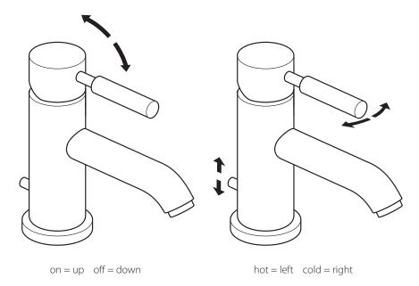
Moving the mixer lever upwards/downwards will increase/decrease the flow of water.
