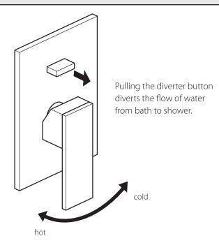
Moving the contol lever anti-clockwise will decrease the water temperature. Pull the handle out to increase the flow of water.
