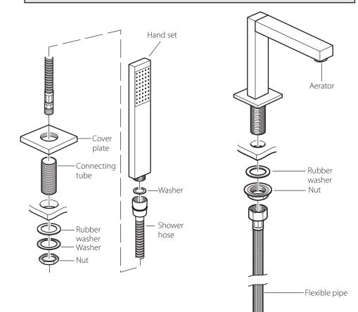
Screw the connecting tube into the cover plate and position in the hole, from the underside slide on the rubber washer, metal washer and then the nut. Tighten the nut to clamp on the cover plate.
