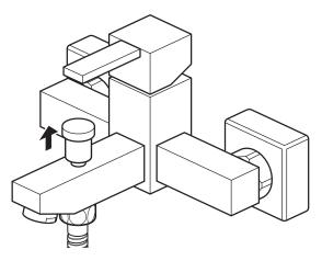
Pull the shower control knob up to turn on the shower, turn to lock in position. Turn back to release and turn off the shower.
