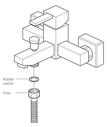
Place a rubber washer into the nut end of the hose and attach it to the mixer outlet.
