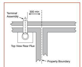
NOTE: The distance from a fanned draught appliance terminal installed parallel to a boundary may not be less than 300mm in accordance with the diagram above, unless the flue deflector kit is used. This can then be reduced to a min of 25mm.
