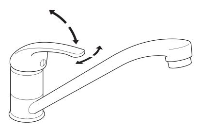
Moving the mixer lever upwards/downwards will increase/decrease the flow of water. Moving the mixer lever from right to left will increase the water temperature.
