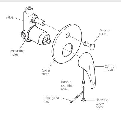
Before installing your new mixer, flush through the pipe work to ensure removal of debris, turn off the water supply.
