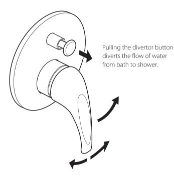
Moving the control lever anti-clockwise will decrease the water temperature.
