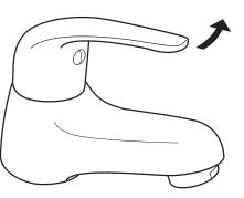
Cold tap - turning the control handle anti-clockwise will increase the flow of water.
