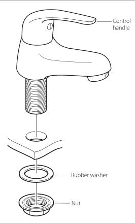
Before installing your new tap, flush through the pipework to ensure removal of debris, turn off the water supply.
