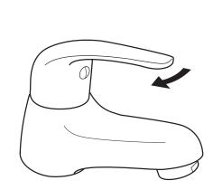
Hot tap - turning the control handle clockwise will increase the flow of water.
