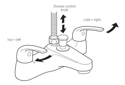
Moving the control handles in the direction of the arrows will increase the flow of water.
