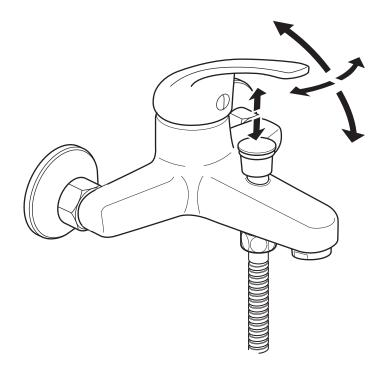
Moving the mixer lever upwards/downwards will increase/decrease the flow of water.
