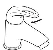
Hot tap - moving the tap lever from right to left will increase the flow of water.
