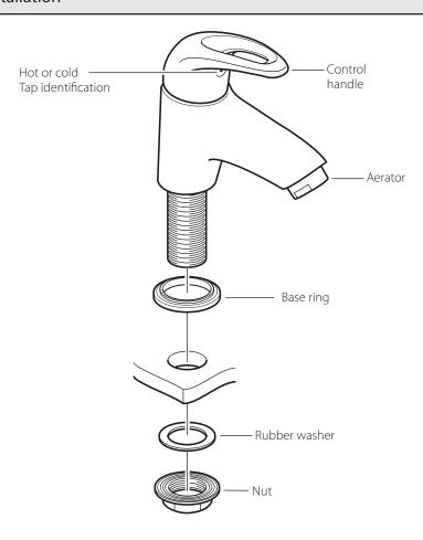
Before installing your new tap, flush through the pipework to ensure removal of debris, turn off the water supply.
