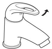
Cold tap - moving the tap lever from left to right will increase the flow of water.
