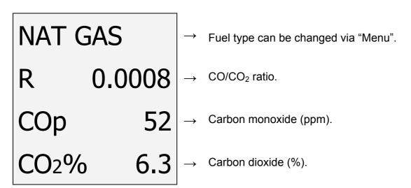
Press Send / to print a full combustion test, (or send to PC via optional Bluetooth).
