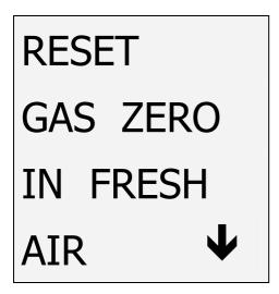
This message indicates that the analyser needs to be reset in fresh air. To do so, ensure that the analyser is in fresh air and press Send / S
