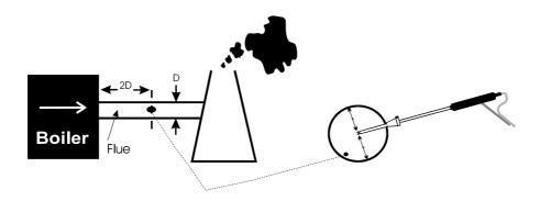
Use the probe's depth stop cone to fix it in flue diameters from  $^{1}/_{4}$  to  $^{4}/_{5}$  inch, 6 to 21 mm. Its maximum operating temperature is 1112°F / 600°C.
