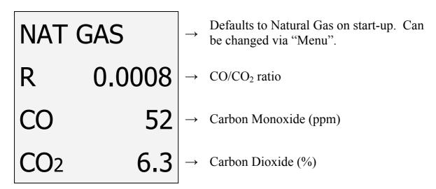
Press Send / to print a full combustion test (also sends to PC if Bluetooth fitted).
